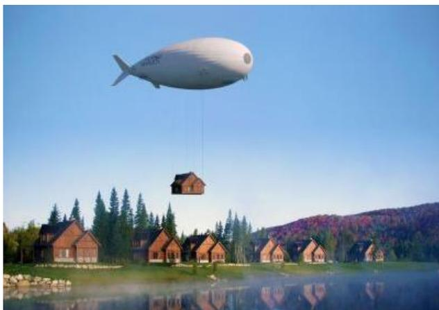
The main advantage of the LCA60T will be its ability to transport heavy and oversized cargo of up to 60 tonnes either in its 75m-long hold or underslung, at speeds of 100 km/h, with a range of several thousand kilometers per day.
